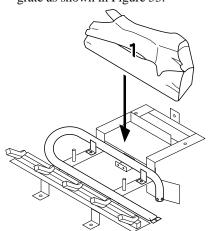
Figure 51 - Installing Log No. 1
